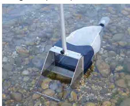
Surber net enabling the sampling of aquatic invertebrates.
